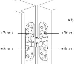
4 b. (For RHS17-120) Vertical adjustment ±3mm. Horizontal adjustment ±3mm.
