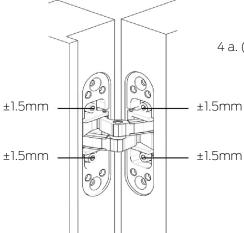
4 a. (For RHS17-80) Vertical adjustment ±1.5mm. Horizontal adjustment ±1.5mm.
